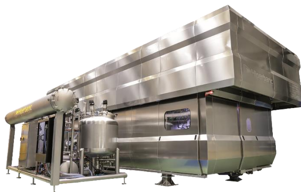
Figure 8: Hiperbaric bulk. Hiperbaric machine model designed specifically per liquids (Hiperbaric S.A.).
